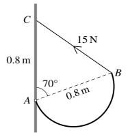
A uniform wire has the shape of a semicircular arc, with diameter AB of length 0.8 m. The wire is attached to a vertical wall by a smooth hinge at A. The wire is held in equilibrium with AB inclined at 70° to the upward vertical by a light string attached to B. The other end of the string is attached to the point C on the wall 0.8 m vertically above A. The tension in the string is 15 N (see diagram).
