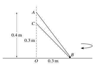
A light inextensible string passes through a small smooth bead B of mass 0.4 kg. One end of the string is attached to a fixed point A 0.4 m above a fixed point O on a smooth horizontal surface. The other end of the string is attached to a fixed point C which is vertically below A and 0.3 m above the surface. The bead moves with constant speed on the surface in a circle with centre O and radius 0.3 m (see diagram).
